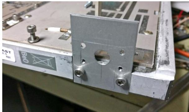
New N connector mounted on baseplate.
