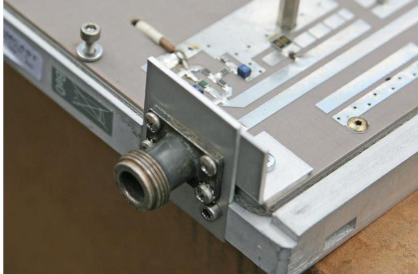
Input BNC and Phono connector mounted on existing block. The original block is steel, hard to machine, but it fits. A bracket could be made from aluminum, or solder cables to vertical shield.
