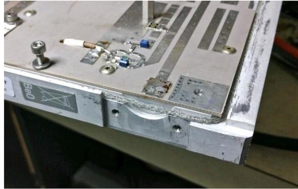
Sheet metal for N conn mount. This mount was made for a N connector with a flat surface on the rear of the mount, this connector happens to be from a Comark TV surplus drawer. With a thicker plate other connectors can be used, Flathead screws would have to be used from the rear to mount the N connector if the screws interfere with the original mounting holes in the cold plate.
