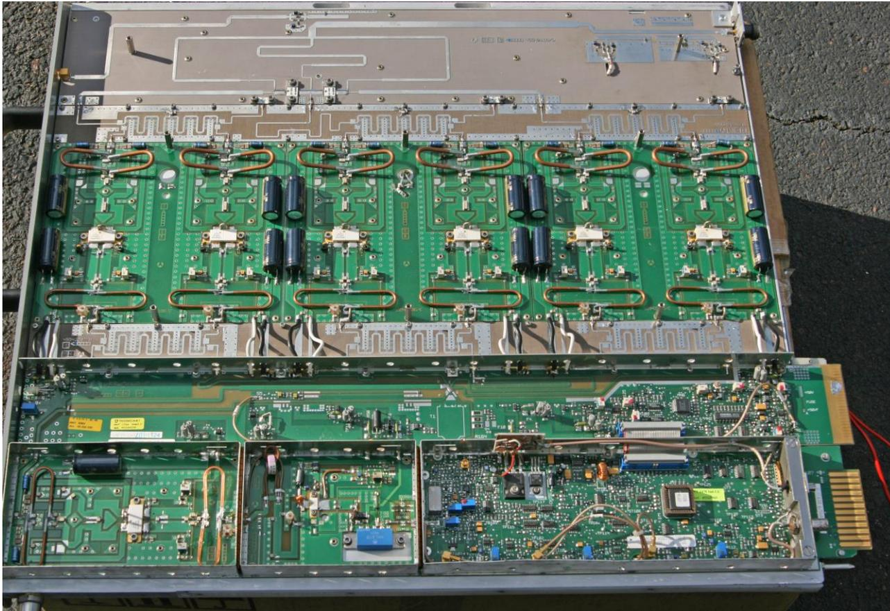
Well designed TV surplus amplifier with many conversion options for use on 222 MHz.
