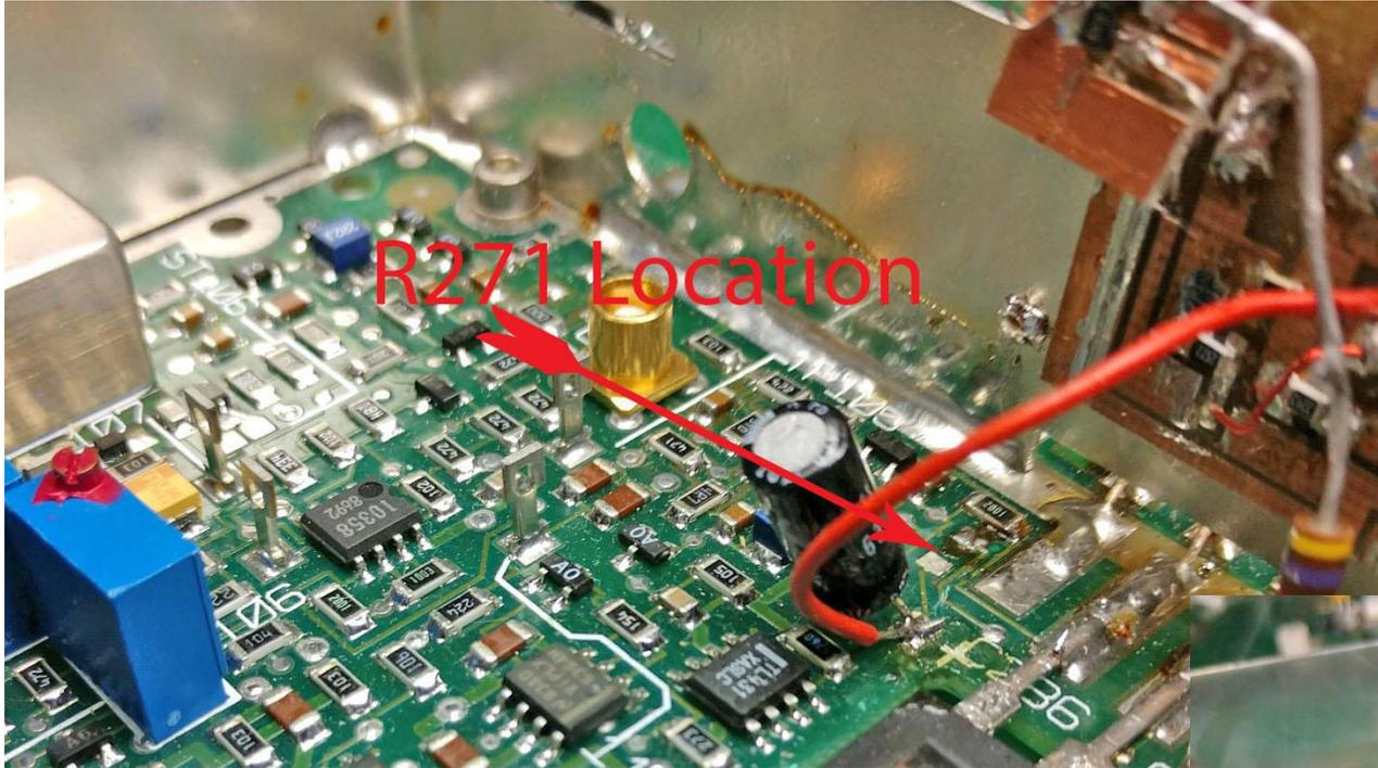
New breadboard prototype bias board, solder or mount on the sidewall.
